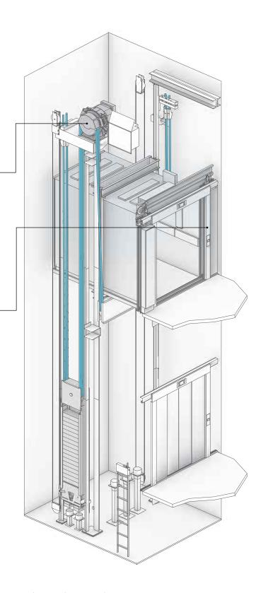
Machine room-less traction elevator
