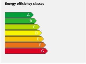
The measurement standard is VDI 4707 established in March 2009 by the Association of German Engineers. Energy efficiency classification can vary depending on elevator configuration.
